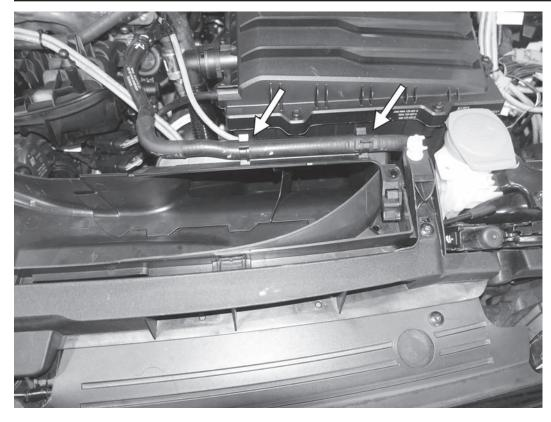
3) Remove the coolant line that runs over the airbox inlet scoop but lifting the coolant line out of the two retaining clips on the scoop.
