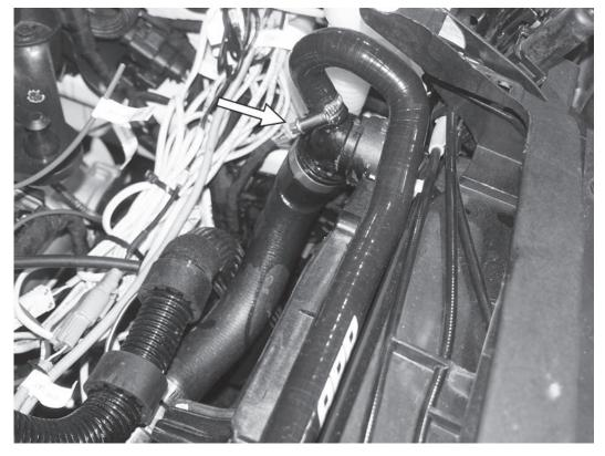
15) Remove the rubber cap from the coolant coupling, and install the APR coolant hose to the coupling, securing it with the bigger, supplied screw clamp.
