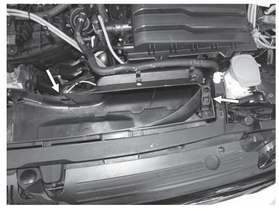
5) Push in the tab on the left side of the airbox intake scoop, and lift off the airbox inlet base. Separate the right side of the airbox intake scoop from the airbox inlet base and remove the scoop from the car. Then, remove the airbox inlet base by pressing in the tab on the right side of the base.
