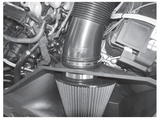
27) Make sure the other end of the APR inlet pipe is fully seated on the flange on the back of the APR airbox. Secure clamps on the APR airbox to 6Nm (53in-lbs).
