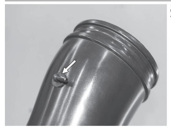
19) Install the supplied 90° barbed fitting into the rubber grommet in the APR inlet pipe.
