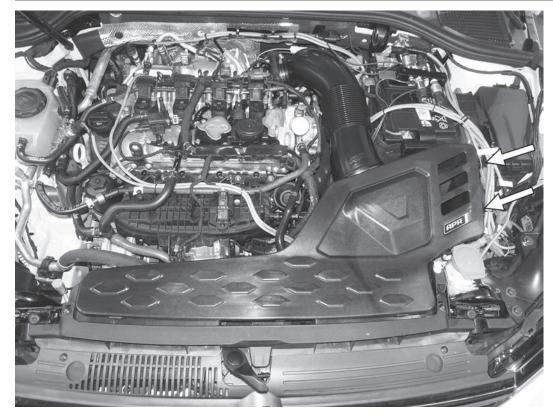
31) Push the APR airbox lid down on the APR airbox. Make sure all tabs snap into place, including the two on the left side of the airbox lid.
