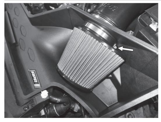
25) Install the APR filter with the supplied clamp onto the inside of the APR airbox. Make sure the filter is fully seated on the flange, and then tighten the clamp to 6Nm (53in-lbs).
