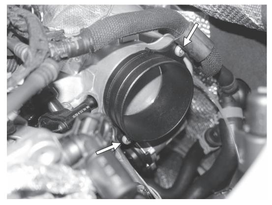
17) Install the APR turbo inlet adapter with the two original T30 screws. Torque the T30 screws to 9Nm (80in-lbs).
