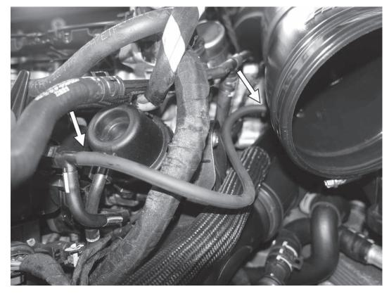
21) Install the supplied vacuum line between the installed port on the APR inlet pipe and the port the factory airbox vacuum line connected to on the side of the intake manifold.
